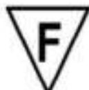
The symbol indicates the suitability of fixtures to be mounted directly on normally inflammable surfaces. Fixtures without the above symbol are only suitable for installation on non-inflammable surfaces.
